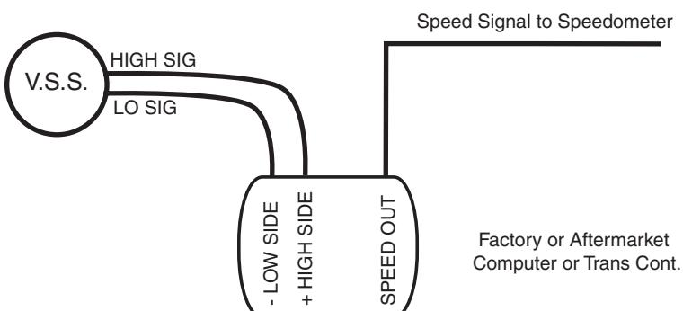
**NOTE:** IF A SPEEDOMETER OUTPUT CIRCUIT IS UNAVAILABLE, OR INOPERABLE, YOU MAY INSTEAD CONNECT TO THE HIGH SIDE SIGNAL. IF FURTHER INFORMATION IS NEEDED, PLEASE CONTACT AUTO METER TECH SUPPORT AT 866-248-6357.
