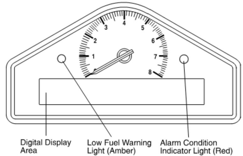
The Display Module is connected to a variety of sensors by a wiring harness. The wiring harness has a 19-way military connector for connection to the Display Module.
