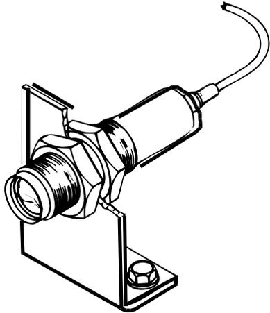
It is secured by two nuts (supplied) with an M18 x 1 mm thread.
