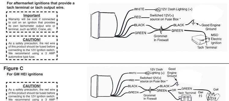
\* Optional: Wire to a switched 12V source with an in line fuse.
