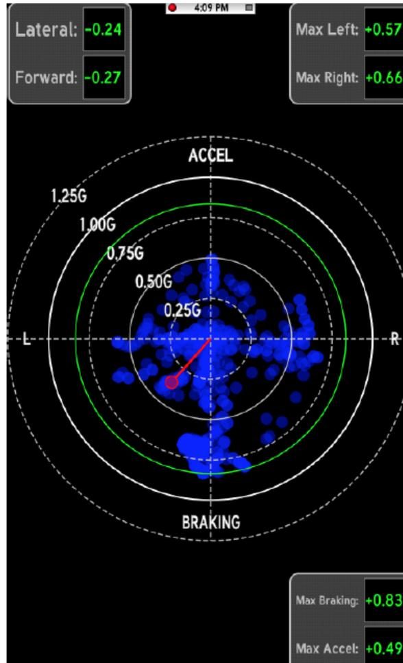
NOTE: Long-holding anywhere on this screen opens a menu with options to Toggle View, Zero the accelerometer, or go back to the Main Menu.
