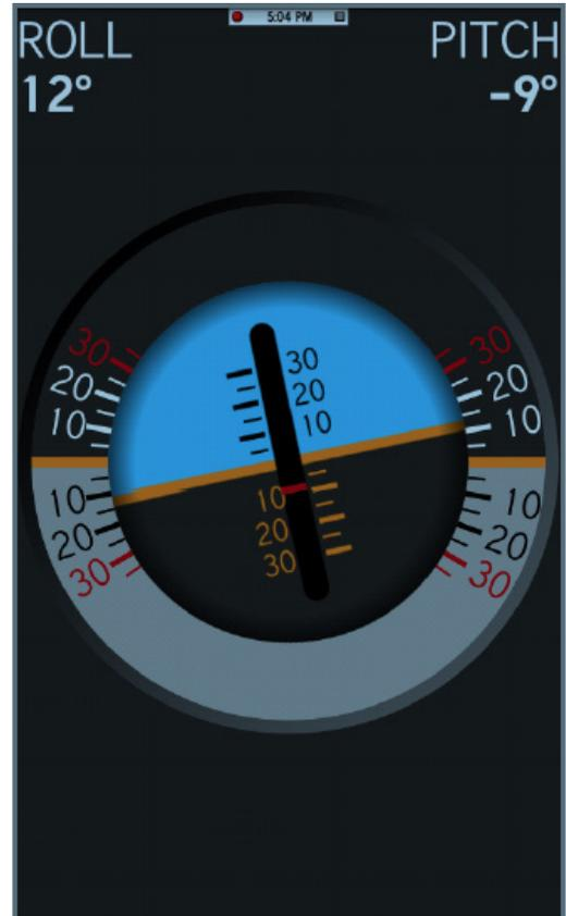
NOTE: Long-holding anywhere on this screen opens a menu with options to Toggle View, Zero the inclinometer, or go back to the Main Menu.
